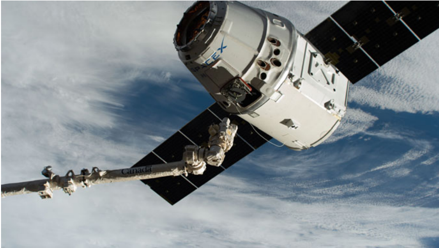
Fig. 23.3 ISS Canadarm2 grapples the SpaceX Dragon. Credits NASA
