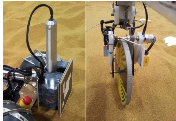
Figure 5- mDCP attached to the scout (left) and WB in front of the primary (right)
