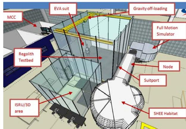
**Figure 3 EAC/DLR artificial analogue concept (:envihab, NBF and big rover testbed not shown)**
