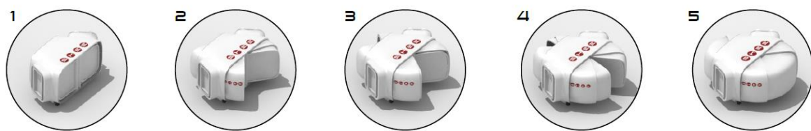
Figure 2: Deployment of SHEE from folded configuration (1) to operational configuration (5).
